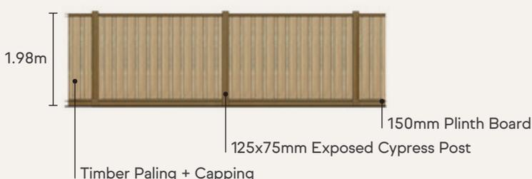
Note: all other internal boundary fencing to be typical maximum 1.98 metre timber fence with capping and exposed post.
